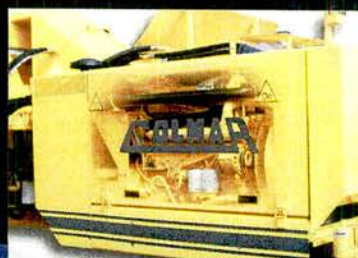
P 5260 Diesel engine and hydraulic pump
