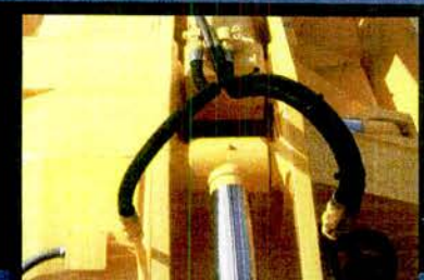
Loading boom arm hydraulic cylinders
